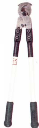
CAT. NO. 704 HEAVY DUTY CABLE CUTTER WITH FIBREGLASS HANDLES Cuts Aluminium and Copper Cables up to 23mm dia. Weight: 1.4Kg Length: 530mm
