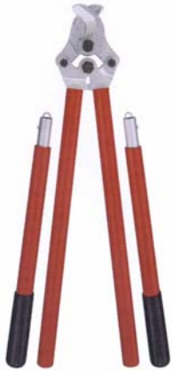
CAT. NO. K101/2 CUTTERS WITH EXTENDABLE HANDLES Cuts Aluminium and Copper Cables up to 38mm dia. Extendable Handles slot in where extra mechanical advantage is required Weight: 4.2Kg Length: 930mm with Handle Extensions
